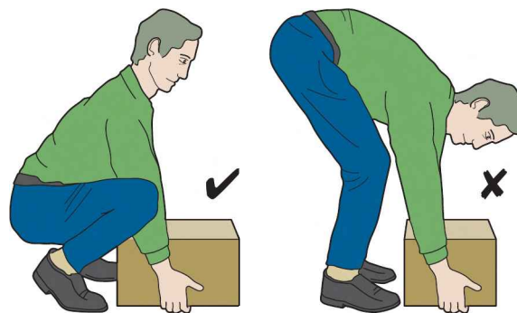
Figure 8.4 Correct and incorrect lifting set-up
